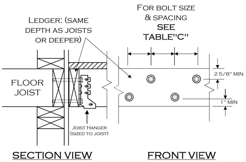
**NOTE:** THIS DECK CONNECTION DETAIL IS BASED ON THE ASSUMPTION THAT A MINIMUM 1-1/2" THICK WOOD MEMBER IS ADEQUATELY INSTALLED AT ALL EDGES OF THE 2ND FLOOR DIAPHRAGM. IF ANY OTHER MATERIAL IS USED, SUCH AS TJI JOISTS, A SPECIAL ENGINEERED DESIGN WILL BE REQUIRED. IT IS THE OWNER'S RESPONSIBILITY TO VERIFY THE PRESENCE OF THE APPROPRIATE RIM JOIST.
