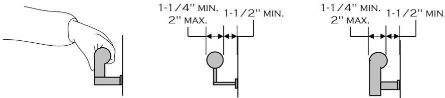
**NOTE: OTHER SHAPES MAY BE ACCEPTABLE IF THEY PROVIDE AN EQUIVALENT GRIPPING SURFACE.**
